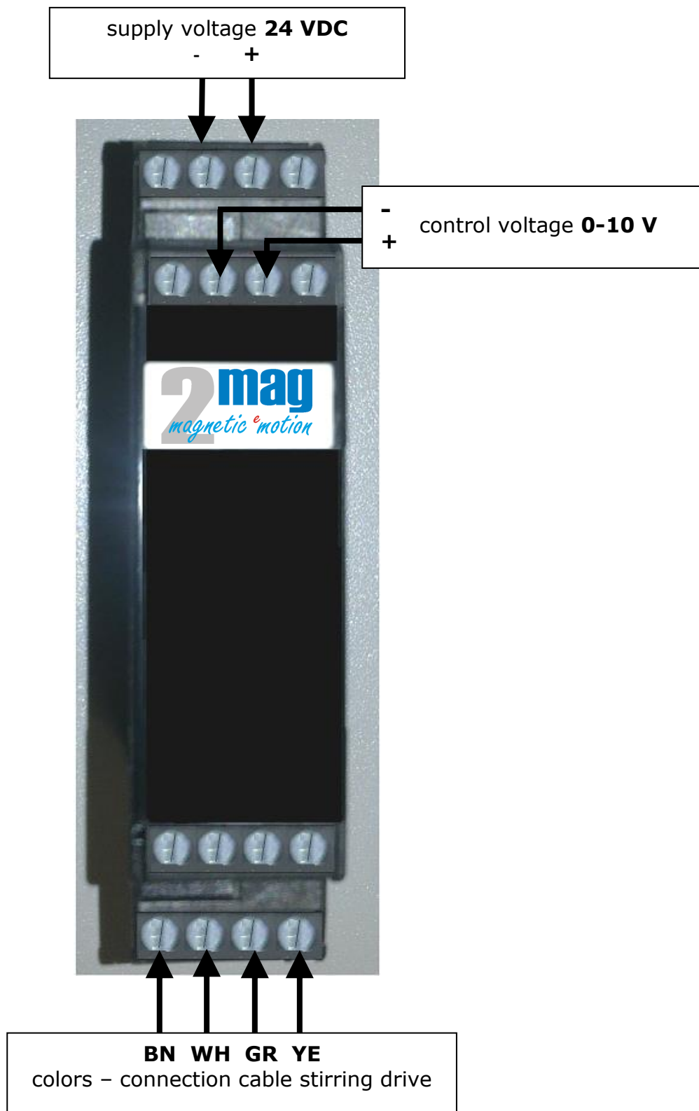
Image 8: Pin-assignment of MIXcontrol eco DINrail 0-10 volts
