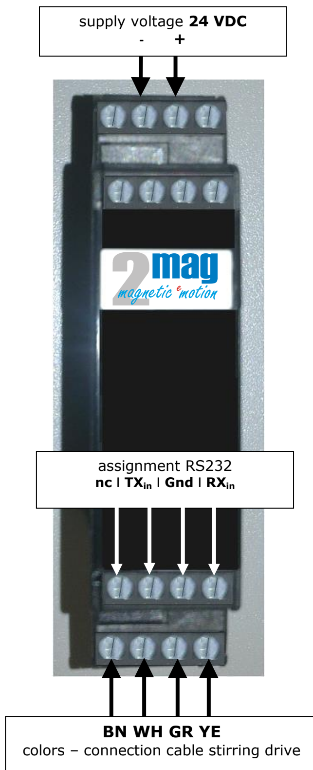
Image 9: Pin-assignment of MIXcontrol eco DINrail RS232
